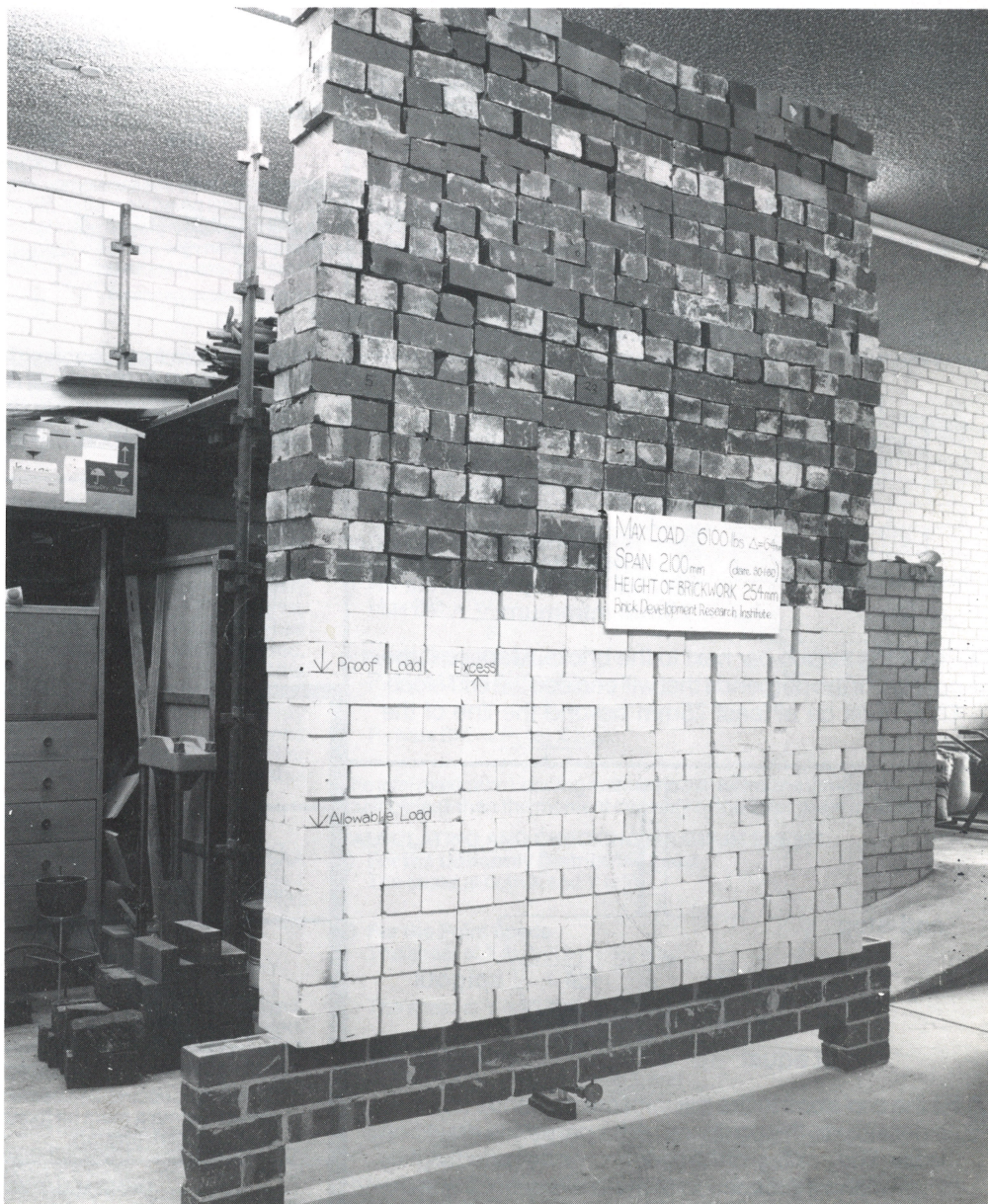
A HESBIA lintel of 2100mm clear span under test at the Brick Development Research Institute. Bricks were used to load the beam to show that long-term creep deflection is small.
